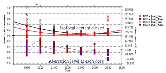
Figure 7: IsoFocal and aberration level response for a comparison of Bottom CD Horizontal (BCDh) and Vertical (BCDv) feature sets.
