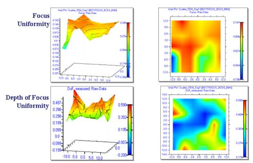
Figure 5: Across-Field critical feature focus and depth-of-focus uniformity
