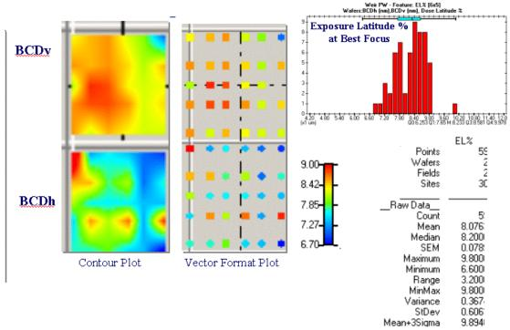
Figure 9: Exposure Latitude Percentage (EL%) uniformity across the reticle for Vertical and Horizontal features. The contour plot on the left is repeated as a 1-D vector plot to it's right. The histogram is a composite of both vertical and horizontal feature sites.
