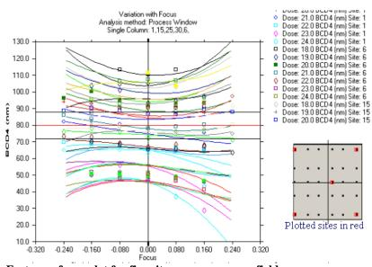
Figure 2: Bossung Feature v focus plot for five sites on an exposure field. This plot illustrates the variation in response to process stimulai when lens and exposure aberrations are present.
