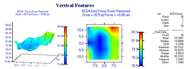
Figure 8: Optimum BCD, Vertical feature response with focus perturbations removed.
