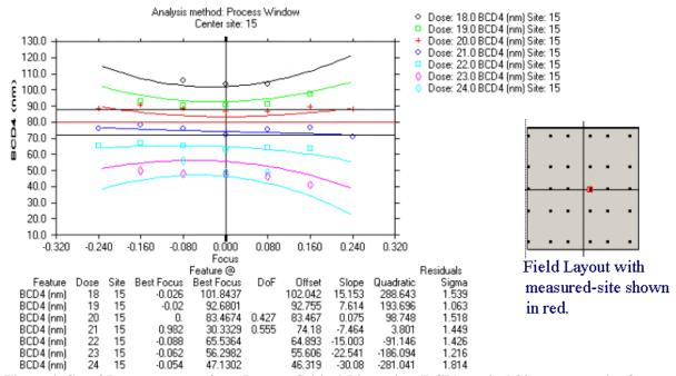
Figure 1: Set of Bossung curves for a Bottom Critical Dimension (BCD) vertical 80 nm target size for one site located in field-center. The analysis shown contains additional information on the Best Focus, feature size and DoF for each curve. (Weir PW software)
