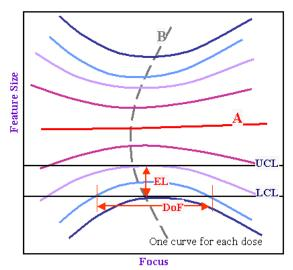
Figure 3: The Anatomy of a Bossung Plot. The response and shape of each dose-curve contains information on the process window and perturbations of the exposure process.
