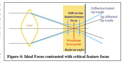
will focus to a single point on the optical axis for the lens. Specialty focus measurement reticles measure focus much somewhat along these lines in an attempt to characterize the optimal wavefront response.
