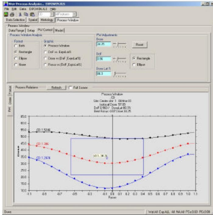
Figure 2: Process window calculation interface.
