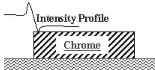
Figure 3: Intensity profile of wavefront at the edge of a chrome knife-edge.
