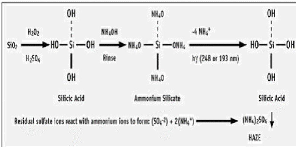
Figure 1: Haze deposition of Ammonium Sulfate (Courtesy Grenon Consulting, Inc.)
