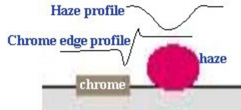
Figure 5: Haze initiation near a reticle feature edge.
