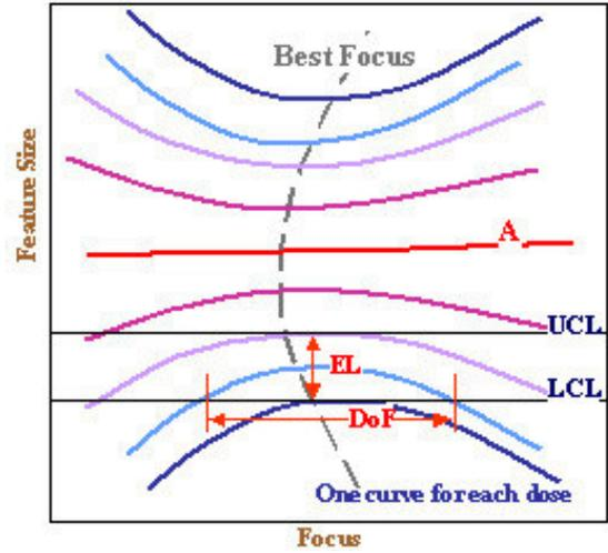
Figure 9: Schematic of Bossung Curve Response
