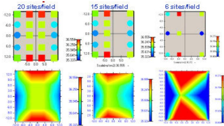
**Figure 8: Hazed-reticle dose uniformity calculated at 20, 15 and 9 metrology sites per field.**
