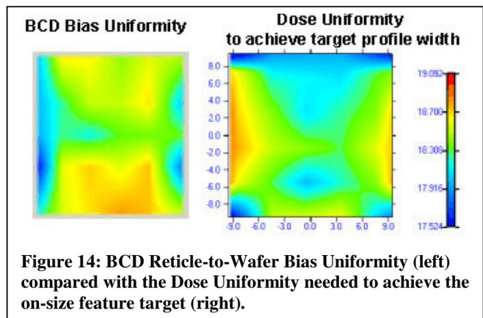
**Figure 14: BCD Reticle-to-Wafer Bias Uniformity (left) compared with the Dose Uniformity needed to achieve the on-size feature target (right).**
