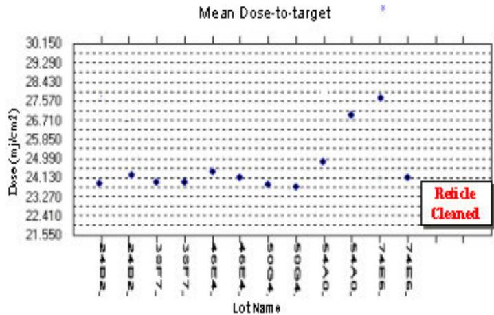
**Figure 13: Trend-plot of the average dose required for feature uniformity on a reticle that exhibited hazing and was subsequently cleaned.**
