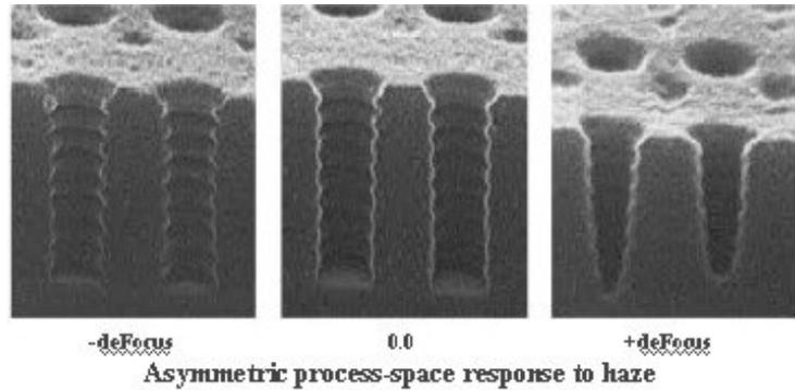
**Figure 7: Haze response to defocus on a via mask**
