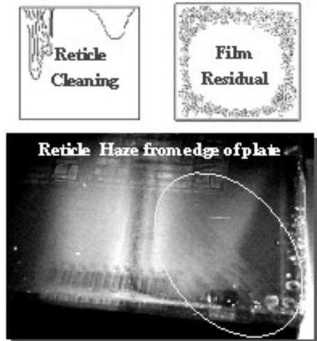
Figure 2: Lower – Haze formations on lower right-side of reticle. Upper – Schematic of two characteristic sources of haze formation
