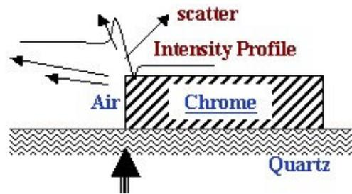
Figure 4: The influence of scatter and finite-chrome thickness on a wavefront.
