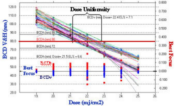
Figure 11: Dose Uniformity plot for a reticle with defocus removal of feature perturbations
