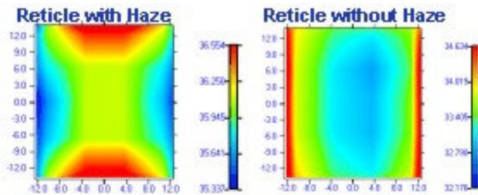
Figure 12: Dose uniformity for a reticle with (left) and without (right) haze contamination.
