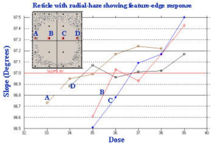
Figure 10: Profile edge-slope for four points on a hazed reticle
