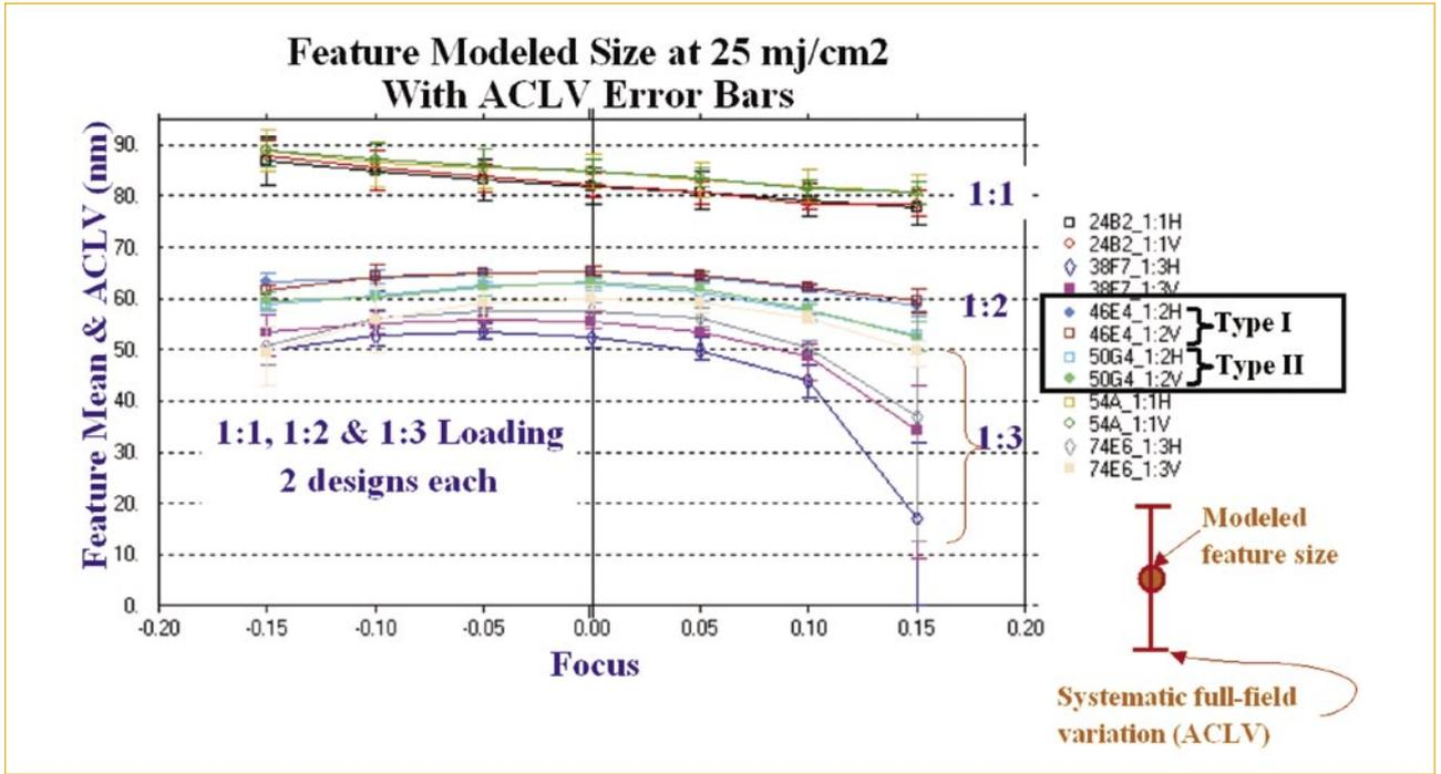
Figure 3. OPC family response to focus with ACLV sensitivity error bars at optimum dose. The results are produced using TEA Systems' Weir PW commercial software.
