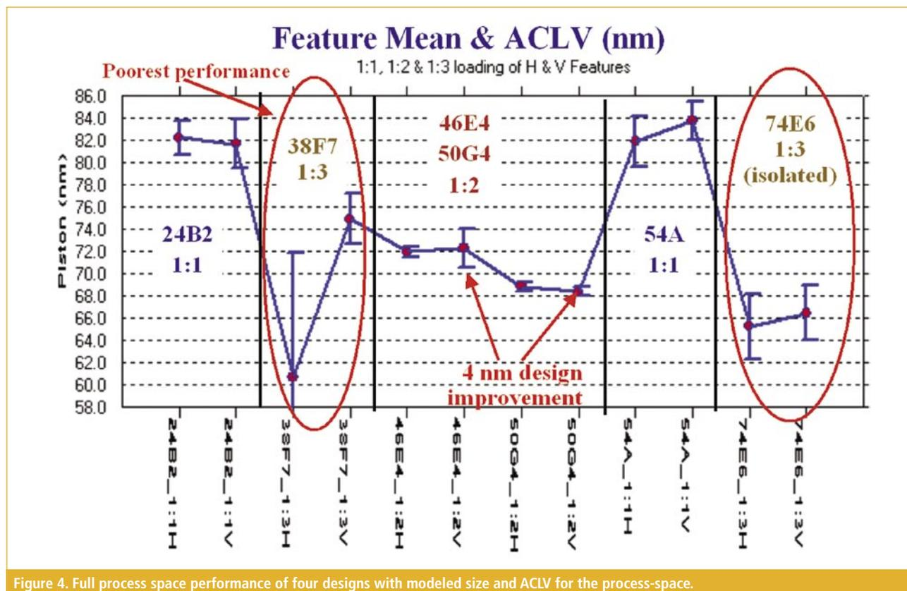
Figure 4. Full process space performance of four designs with modeled size and ACLV for the process-space.
