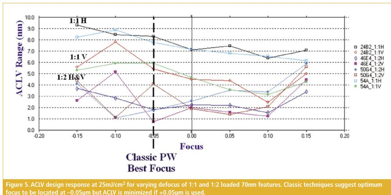
Figure 5. ACLV design response at 25mJ/cm<sup>2</sup> for varying defocus of 1:1 and 1:2 loaded 70nm features. Classic techniques suggest optimum focus to be located at  $-0.05\mu\text{m}$  but ACLV is minimized if  $+0.05\mu\text{m}$  is used.
