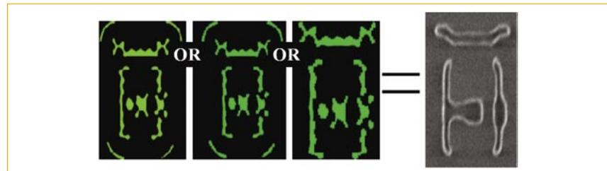
Figure 2. Three design alternatives for an SRAM gate binary mask pattern. Design, simulation and wafer.
