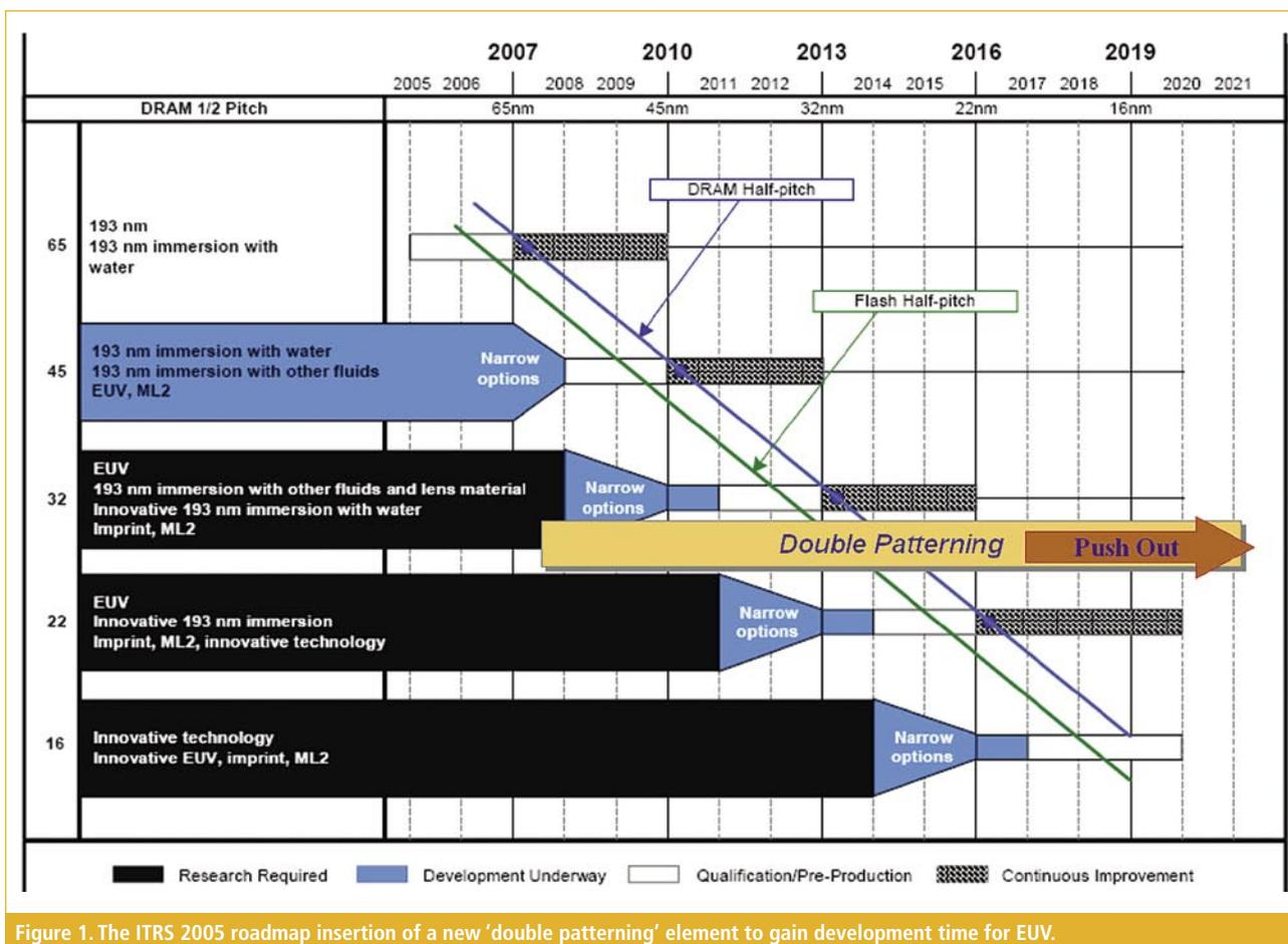
Figure 1. The ITRS 2005 roadmap insertion of a new 'double patterning' element to gain development time for EUV.
